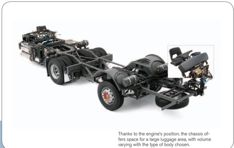
Thanks to the engine's position, the chassis offers space for a large luggage area, with volume varying with the type of body chosen.
