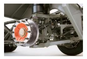
All the wheels have disc brakes with EBS, electronic control and ABS.
