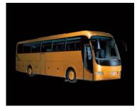
Rear-mounted engine permits low floor height and at the same time offers considerable flexibility in the design of the finished bus.
